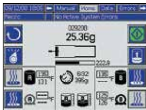
Recirc Mode option prevents materials from setting overnight
