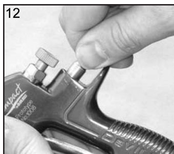
12. Fit Valve Seat to Gunbody.
