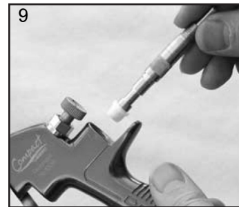
9. Fit New Front Seal to Service Tool.
