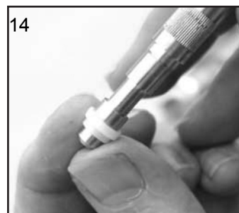
14. Fit new Seal to Service Tool.
