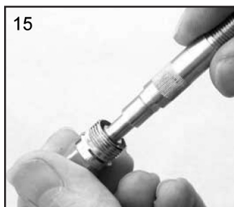
15. Fit Seal to Housing (10).
