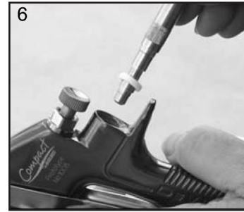
6. Remove Valve Seat.
