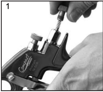
1. Remove Adjusting Knob (7), Spring (8), and Needle (9).
